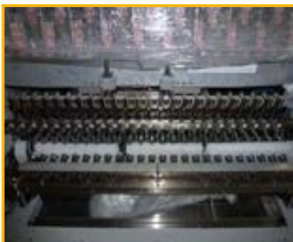
Bobbin Support: Reduce To Deform After Winding Or To Hold Special Shape Bobbins
