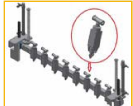
Cutter : Cutter For Thick Wire Over 0.28mm Diameter
