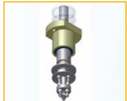
Wire Polish: For Wire 0.2 To 0.7mm To Remove Enamel
