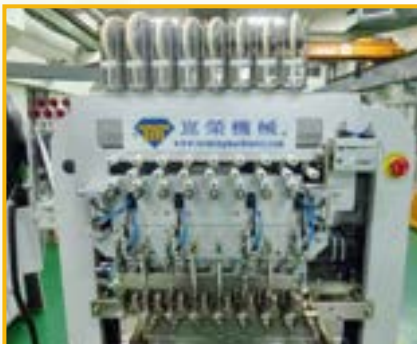
Taping: Interlayer Taping From 3 To 25mm Tape Width
