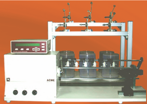
Six Coil Winder with AEX mechanical and control unit
